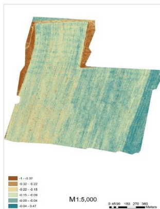
Figure 8. Three-dimensional drawing of the soil surface A three-dimensional model of the surface was made using drone aerial mapping data.
