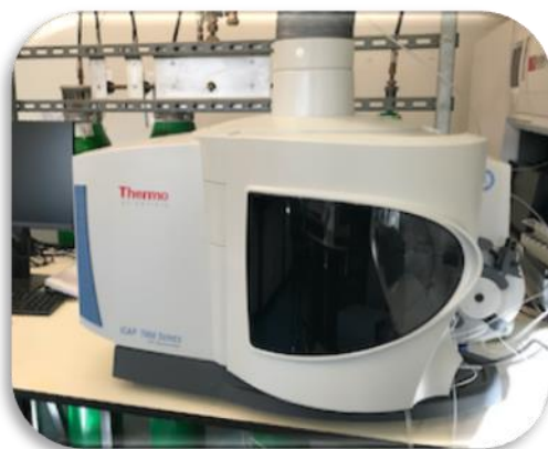
iCAP-7400 ICP-OES (Inductively Coupled Plasma-Optical Emission Spectrometry)
