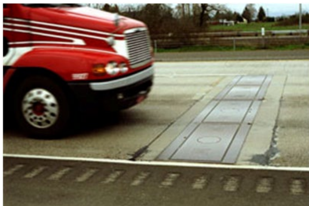
Figure 13 Wheels over a plate and a strip sensor
