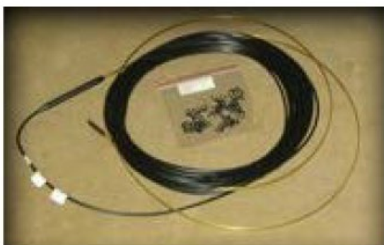
Figure 2.2 Measurement Specialties Roadtrax BL piezoelectric sensor
