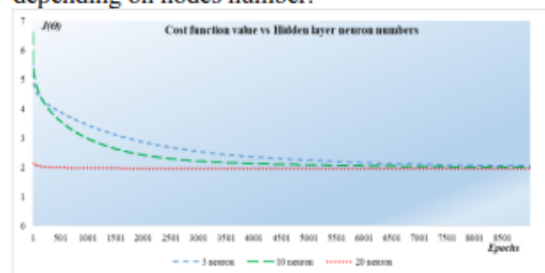
Fig. 6. Dependence of Cost function value and node numbers.
