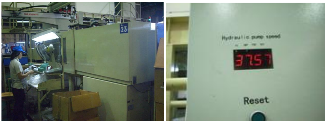
Plastic Injection Molding Machine and Inverter for Hydraulic Pump
