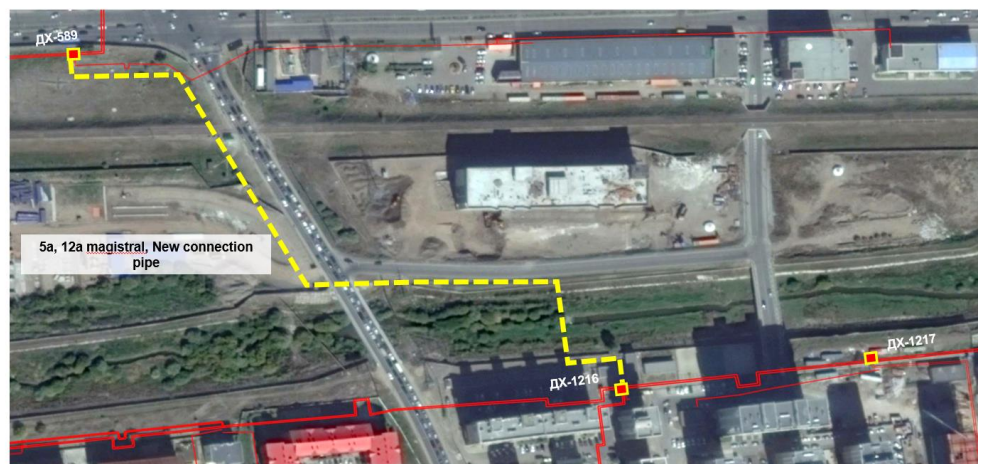
Connection pipe network between 5в-12a magistral
